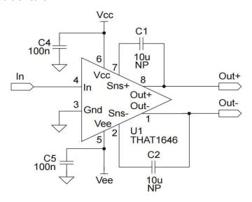
The practical schematics is recommended by THAT and we use this on our BoutLin-1646 module. Actually it's just the IC, completed with some decoupling capacitors and power supply parts.
