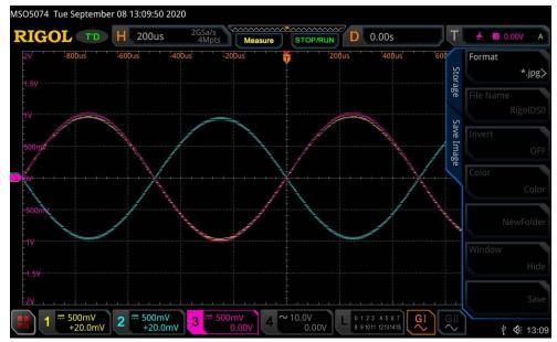
LinBout-1646 running at 1kHz/1V,  $0^{\circ}$  phase shift from input to + output. Yellow is +out ( $0^{\circ}$ ), Blue is -out ( $180^{\circ}$ ), Magenta is input signal.
